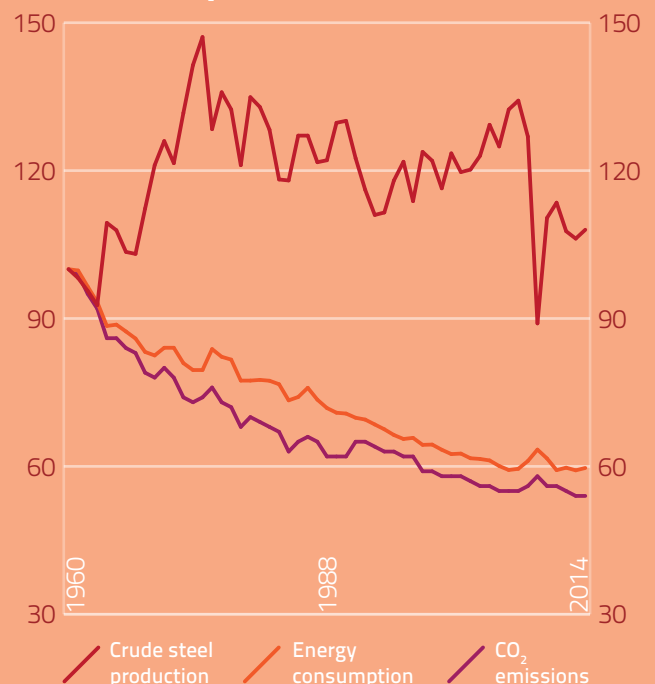
Index of crude steel production, specific energy consumption and specific CO 2 emissions compared to 1960 (=100)
